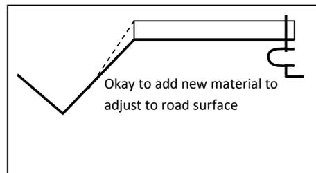
If it is necessary to increase or widen shoulders contact the REC for assistance. Shoulder widening can involve a permit from the Corps of Engineers. Activities that require Corps permits are outside the scope of the Blue Book. Widening or increasing the shoulder has the potential to impact archaeological sites and/or change site hydrology, ditch hydrologic capacity, and stream dynamics.
